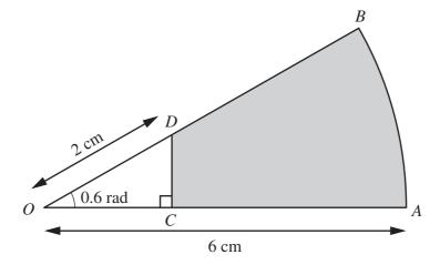
The diagram shows a sector AOB of a circle with centre O and radius 6 cm. Angle AOB = 0.6 radians. The point D lies on OB such that the length of OD is 2 cm. The point C lies on OA such that OCD is a right angle.
