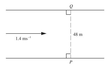
The diagram shows a river with parallel banks. The river is  $48 \,\mathrm{m}$  wide and is flowing with a speed of  $1.4 \,\mathrm{ms}^{-1}$ . A boat travels in a straight line from a point P on one bank to a point Q which is on the other bank directly opposite P. Given that the boat takes  $10 \,\mathrm{seconds}$  to cross the river, find
